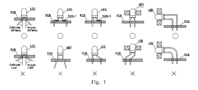
" $\circ$ " Correct mounting method " $\times$ " Incorrect mounting method
