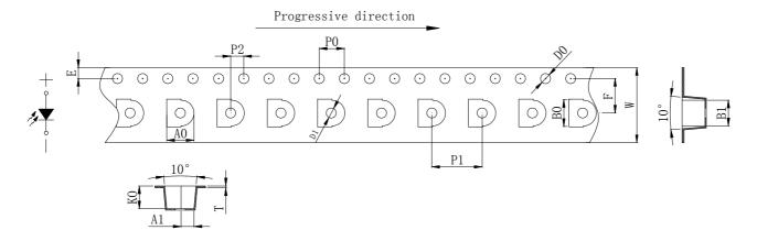
**Note:** Tolerance unless mentioned is  $\pm 0.1$ mm; Unit = mm
