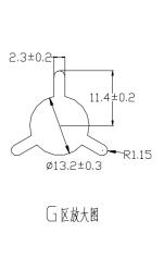
**Note:** Tolerance unless mentioned is  $\pm 0.2$ mm; Unit = mm
