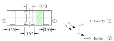
For reflow soldering(propose)
