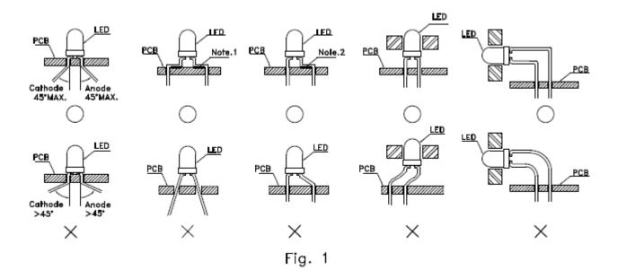
"o" Correct mounting method "x" Incorrect mounting method
