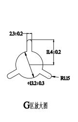
**Note:** Tolerance unless mentioned is  $\pm 0.2$ mm; Unit = mm
