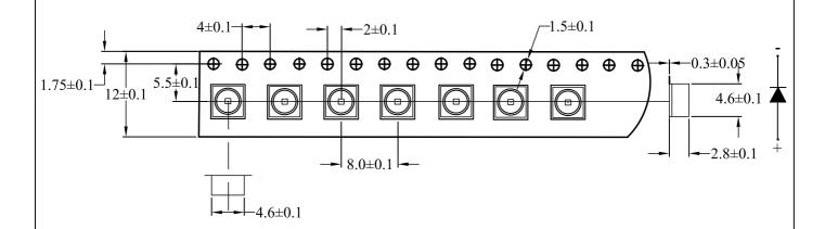
**Note:** Tolerance unless mentioned is  $\pm 0.1$ mm; Unit = mm
