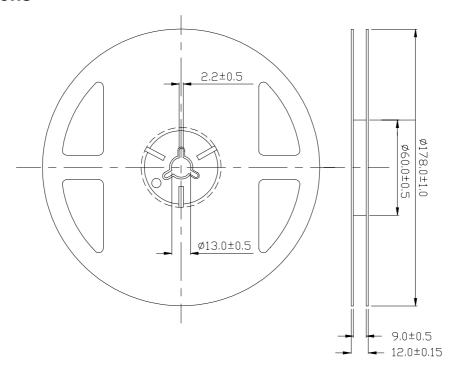
**Note:** Tolerance unless mentioned is  $\pm 0.2$ mm; Unit = mm
