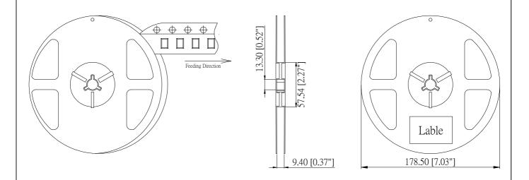
**Note:** Tolerance unless mentioned is  $\pm 0.2$ mm; Unit = mm
