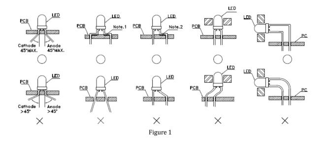
" $\circ$ " Correct mounting method, "×" Incorrect mounting method, Note 1-2:Do not route PCB Trace in the contact area between the leadframe and the PCB to prevent short-circuit.
