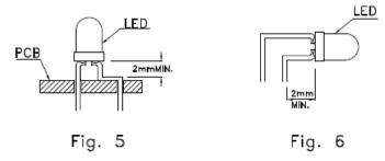
2. Lead forming or bending must be performed before soldering, never during or after soldering.
