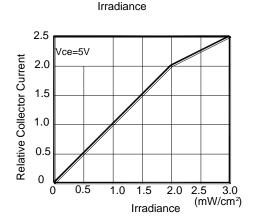
FIG.4 Relative Collector Current Vs.
