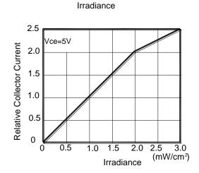
FIG.4 Relative Collector Current Vs.
