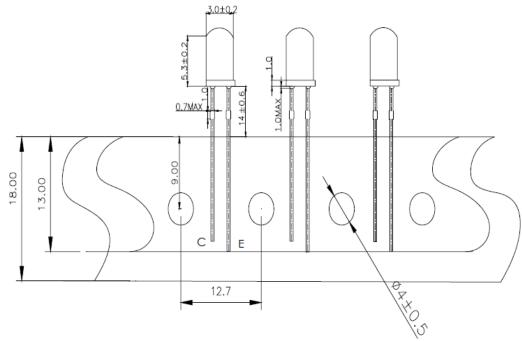
All dimensions are in millimeters. Tolerance is ±0.20mm unless otherwise noted.
