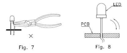
6. After soldering or other high-temperature assembly, allow the LED to cool down to  $50^{\circ}$ C before applying force (Fig.9). In general, avoid placing excess force on the LED to avoid damage. For any questions please consult with LIGHT representative for proper handling procedures.
