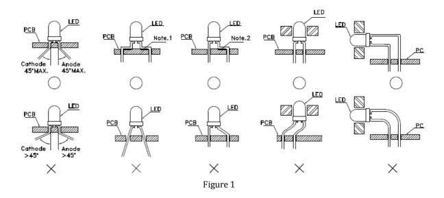
"o" Correct mounting method, "x" Incorrect mounting method, Note 1-2:Do not route PCB Trace in the contact area between the lead frame and the PCB to prevent short-circuit.
